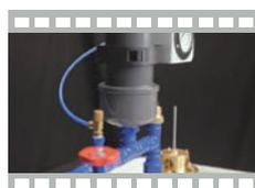
A compact experiment for use with the Hydraulic Bench (H1F) to demonstrate the use of water hammer to create a pumping action.
