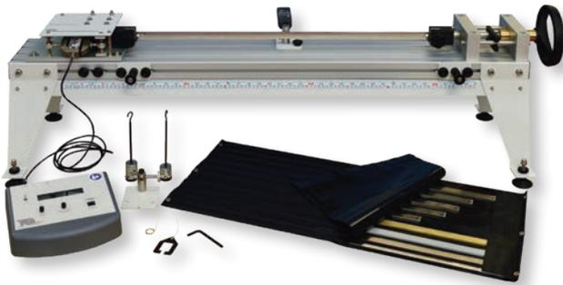
Benchtop apparatus tests different types of struts and demonstrates how they deflect under load, and demonstrates the use of Southwell's method. Set of additional struts available.
