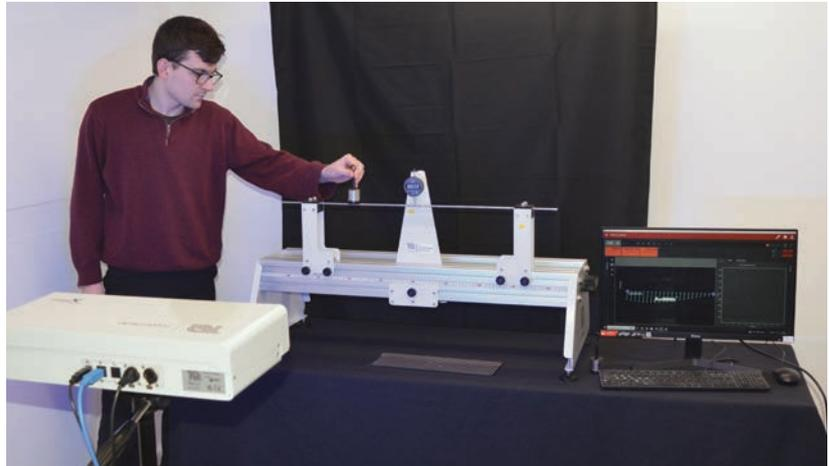
Deflex® is a contactless digital technique to help students learn how to measure and analyse deformations of objects optically. It is equipped with camera measurement and image processing software for analyzing motions, displacements and strains. It can measure visible features on objects and material surfaces like screws, joints, edges, grooves and composite structures.
