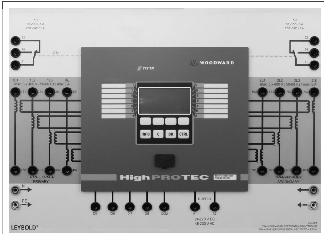
Fig. 16: Transformer differential protective relay
